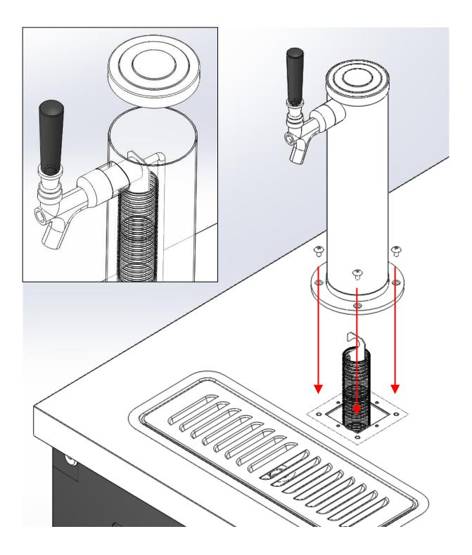
**Beer Line & CO<sub>2</sub> Line Installation Schematic Diagram**
